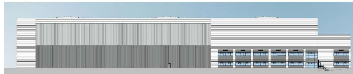
Features such as windows, doors and solid walls should create vertical and horizontal rhythms along the façade providing variety
