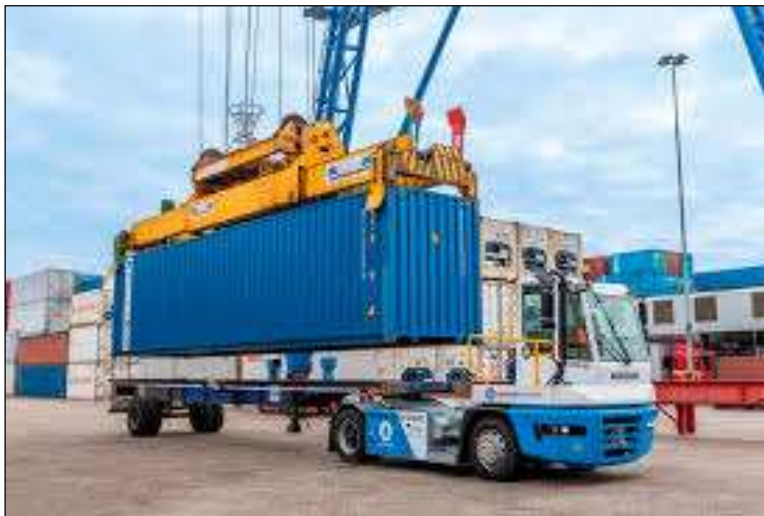
Picture 1: Yard Tractor and Semi-trailer
