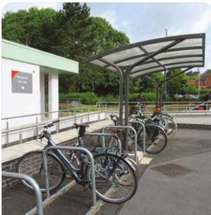
Sheffield stands and shelter, Leamington
