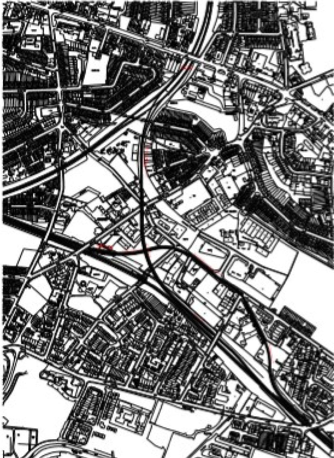
Proposed arrangement at Soho Pool. Metro diverted (a cutting and a road running section) to allow the new link railway to cross over Metro to join the railway to Walsall
