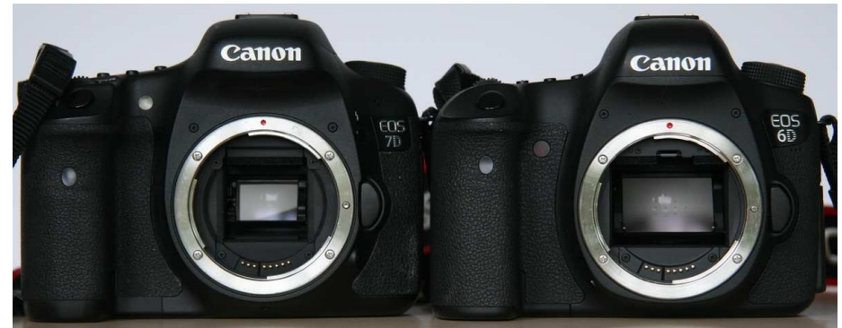
Fig A1.1 Illustration of Cropped-frame and Full-Frame Sensors (FFS): Canon 7D (cropped APS-C, left) and 6D (full-frame, right)
