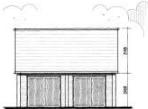
Garage North Facing Elevation Scale 1:100
