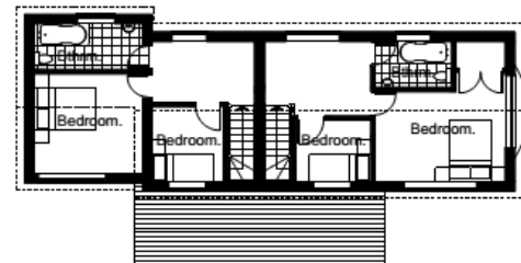
Proposed first floor plan.
