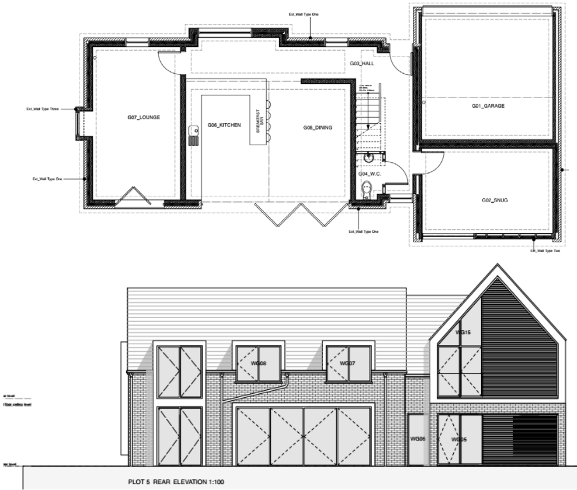
No. 5 ground floor and rear plans from planning consent PAP/2013/0288 showing primary window positions.
