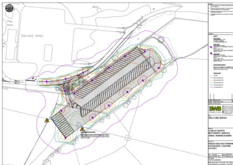
Figure 2: Lighting Layout Plan for approved HGV Park.
