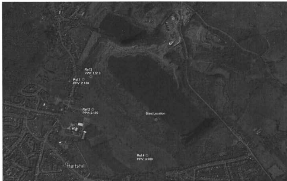
Figure 4: Site Visit, 17.07.2019, Recorded Results
