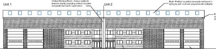
Front Elevation - Units 1 & 2
